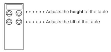
Press LINE 2 on the controller panel ▲ ▼ to adjust the tilt of the table.
